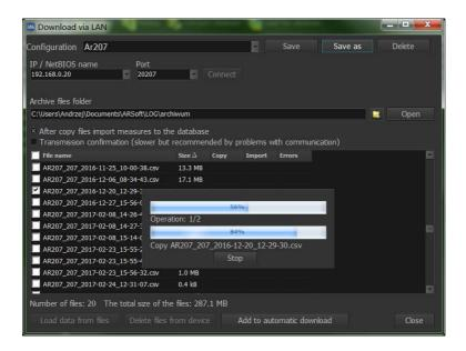
In order to establish communication, enter the IP address (or Netbios name) and the UDP port, then press *Connect*. With more recorders you can save the connection configuration for each device and then select it from the list. You can also select the folder where the downloaded files will be locally archived.
