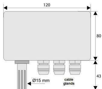
**b) dimensions for external probes in different designs**b.1) AR247/2
