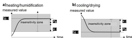
In order to avoid unnecessary activation of tuning, which may slow down the process, it is recommended to set the highest possible value of **Hd**, not less than 10-30% of the range of variability of the process (the temperature or the humidity). Testing of the object with temporary switchoff of the output and the **Run** message also takes place in the insensitivity band if sudden changes in the measured value or preset value are detected.
