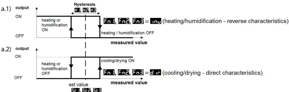
b) additional operating characteristics of outputs (applies only to outputs 2 and 3)
