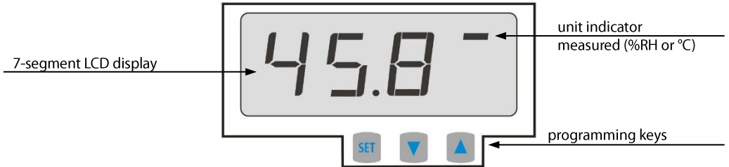
Fig. 8. Description of the control panel
