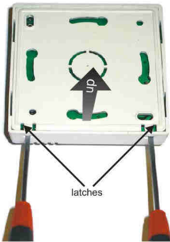
Fig.13.1. Disassembly of the rear wall
